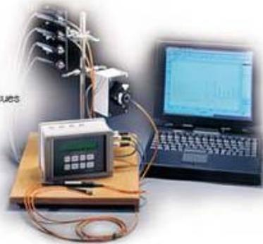
The Walz Company markets a variety of units to determine productivity of plants in terrestrial settings and submerged to 50 m. The field versions of this equipment are extremely light and compact. The methodology is completely non-invasive, and readily lends itself to repetitive measurements on the same plant or leaf over time.
