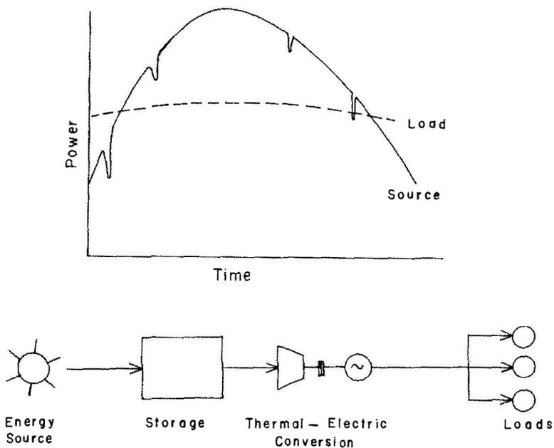
FIGURE 1. Characteristics of Storage System for Intermittent Source
