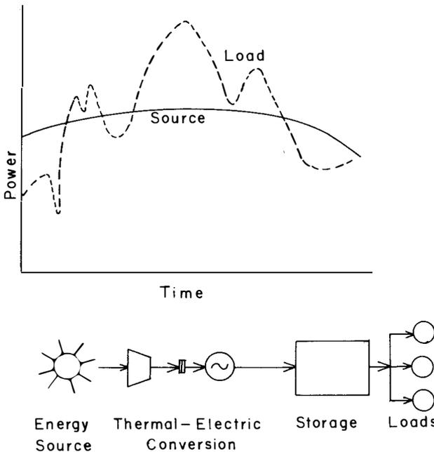
FIGURE 2. Characteristics of Storage System for Intermittent Load
