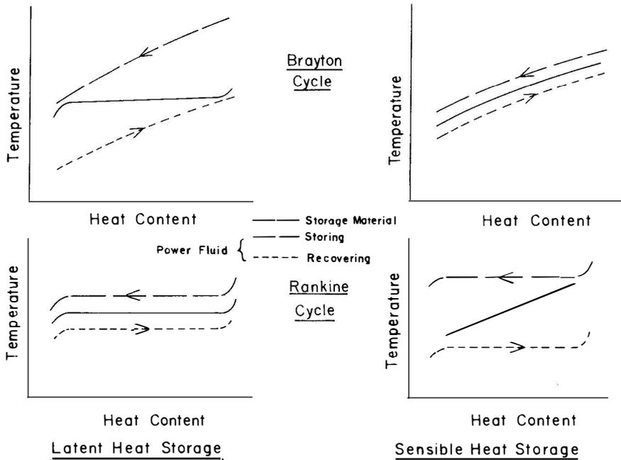
FIGURE 3. Matching Type of Storage System to Type of Power Conversion System
