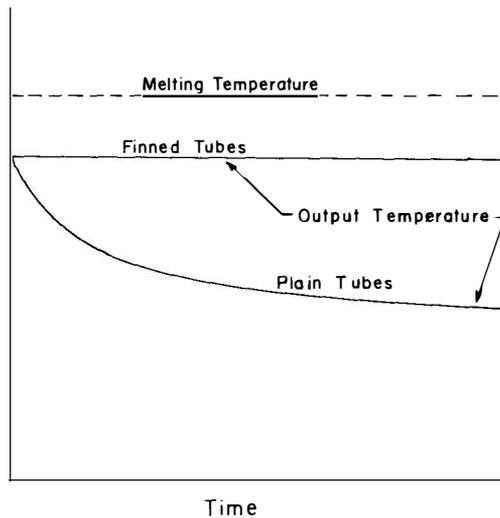
FIGURE 4. Performance of Latent Heat Storage Units with and without Finned Tubes
