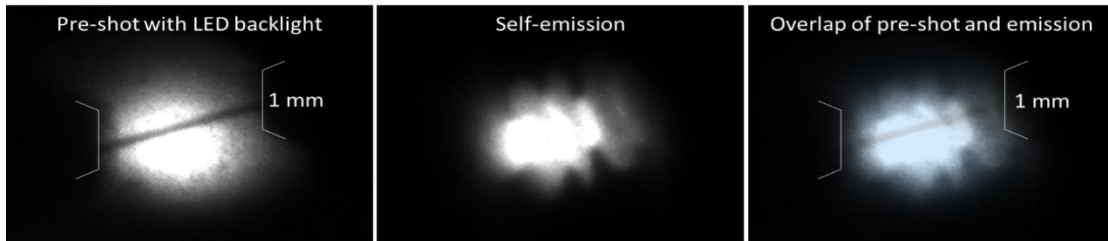
Figure 3.22 Images from a molybdenum hybrid x-pinch on Mykonos. Pre-shot (left), self-emission (center) without a backlight, and a simple overlap of the two (right). The overlap image was created by placing the pre-shot image at 60% transparency over the emission image from the shot. The wire is \sim 100 \mu\text{m} in diameter with a nominal 2 mm gap between the cone tips.
