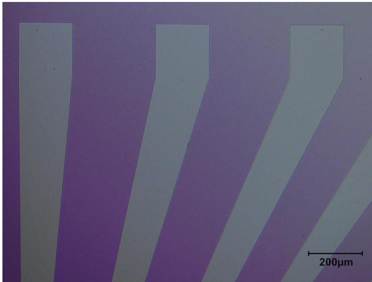
Figure 4.121: Sixteenth generation memristor, post ion mill. The metal in the top right corner is not fully milled as it lay at the outer radius of the ion beam.
