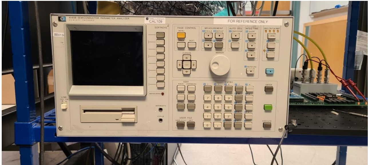
Figure 4.84: HP 4145B Semiconductor Parameter Analyzer connected to PCB [Credit: Landon Schmucker 2021].
