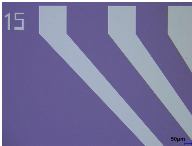
Figure 4.118: Sixteenth generation memristor, bottom electrode lithography.
