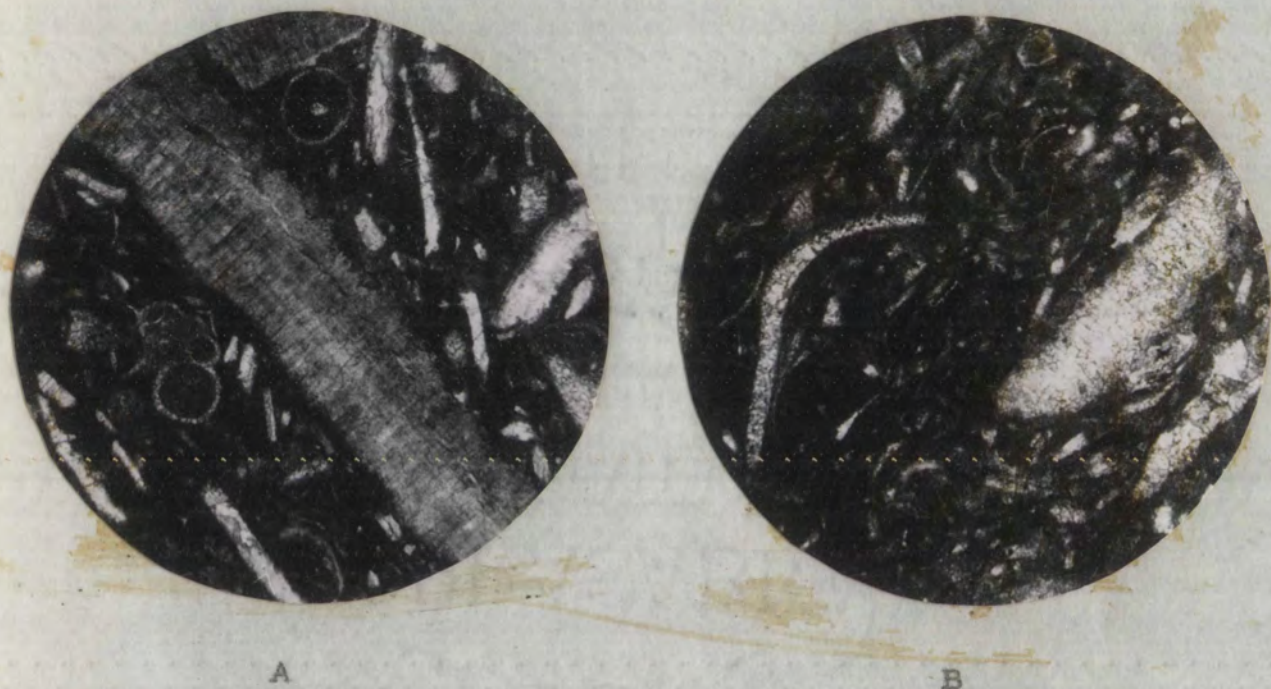
Figure 10. Biomicrites from the brachiopod-bryozoan limestone unit as observed in (A) the lower angular fossil fragment zone, and (B) the upper rounded fossil fragment zone. Crossed nicols, X 22.
