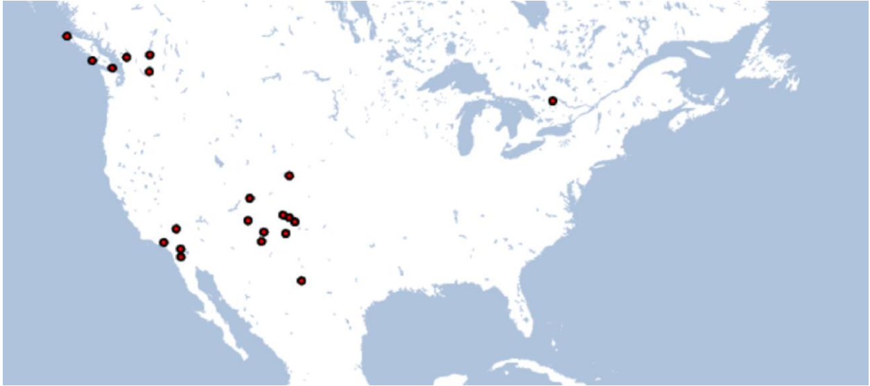
Figure 15. A map showing the locations of all IGS sites used in the GPS processing. Map created using Generic Mapping Tools.
