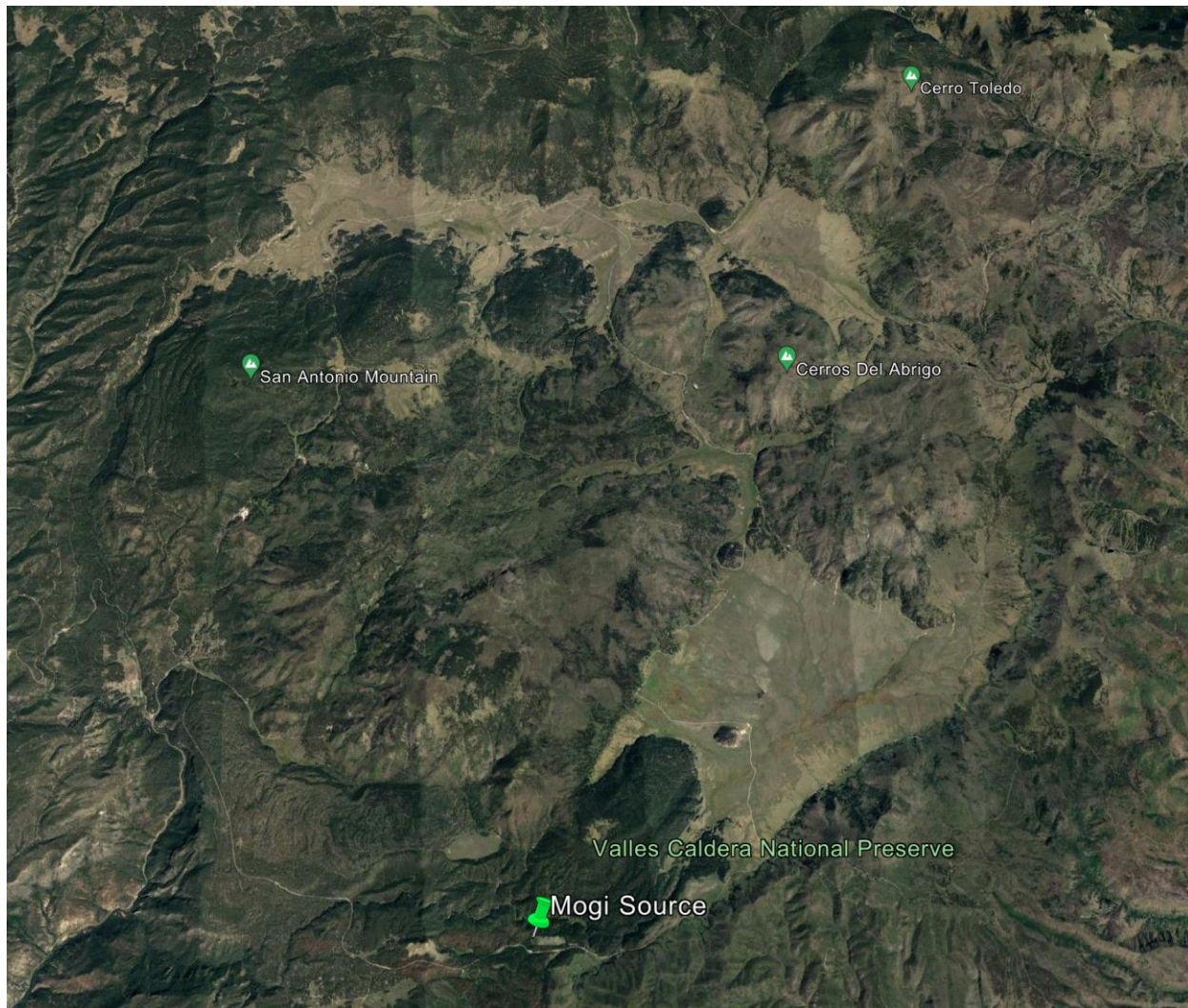
Figure 24. The location of the best-fit Mogi source. This is closest to the station “CNCH,” which has the highest rate of subsidence in the GPS observations.
