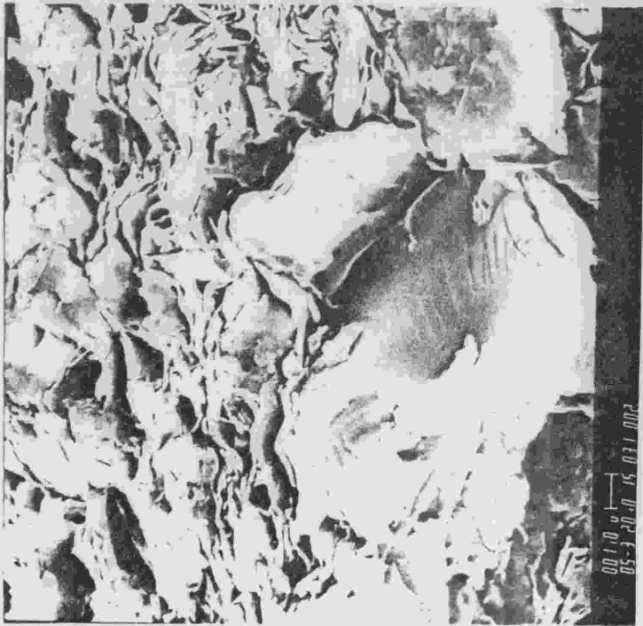
A. Slab-shaped detrital grains may have less disruptive effects on allogenic clay fabrics than spherical grains (5000X).
