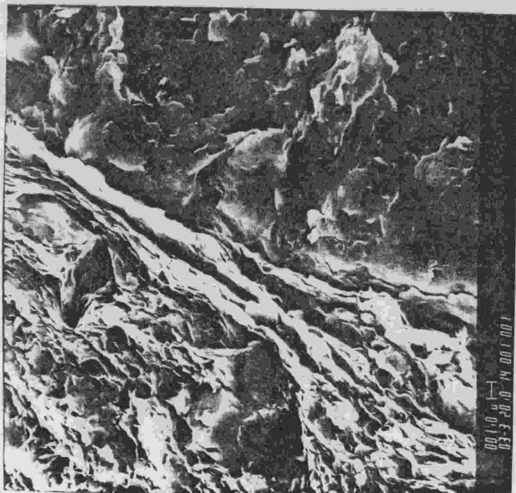
A. Flowage of allogenic clays parallel to grain surface; the partings in the clay laminae adjacent to the grain boundary may be pore-fluid channels (3000X).
