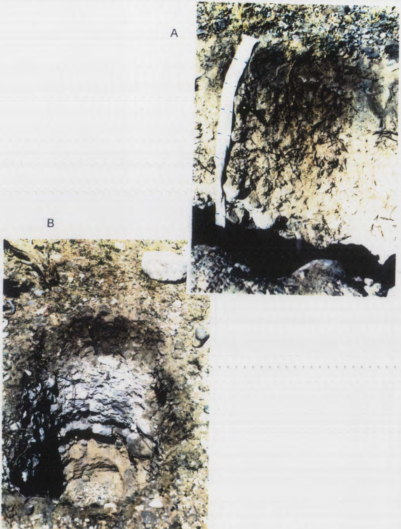
Figure 22. Photographs of the Ash soil. A) Soil pit 9 on the Ash terrace. The only organic-rich A horizon observed in any of the soil pits is seen at the top of this profile beneath a 5 cm thick Av horizon. The entire profile effervesces in dilute hydrochloric acid, but percent carbonate is relatively low (table 4). Graduations on tape are 10 cm apart. B) Soil pit 4 on the Ash surface. This view exposes a profile much like that in 22A, and also shows the weakly cemented Bk3 horizon at the base of this pit. Note knife for scale.
