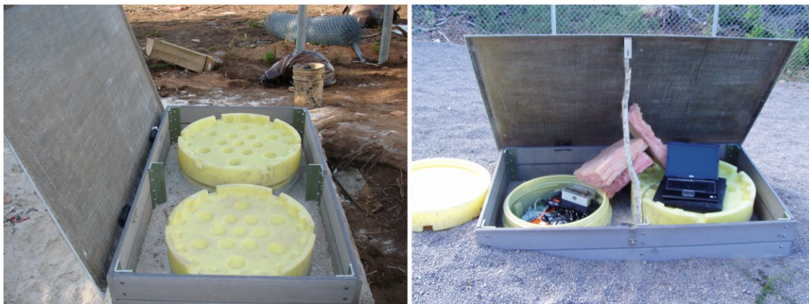
Figure S1. Photographs of station ANWB showing small footprint vault installation style.
