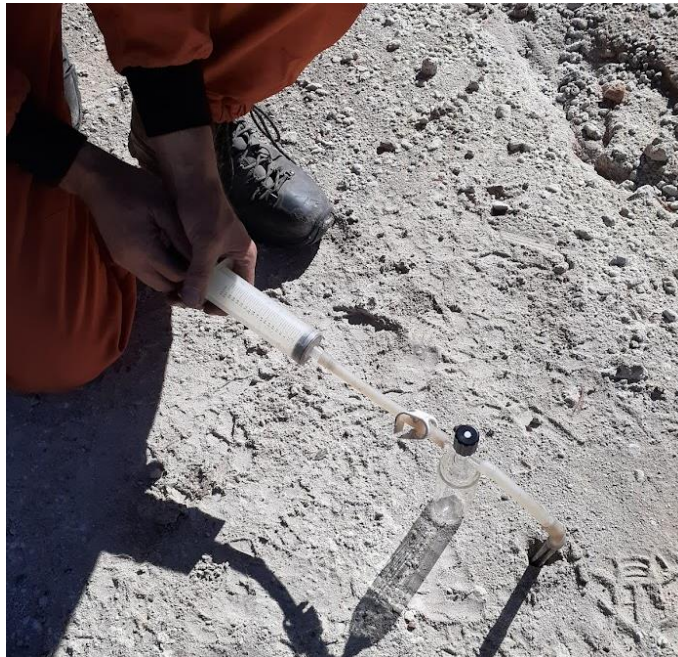
Figure 3.2: Using a syringe to collect a soil gas sample at a depth of 40 cm.
