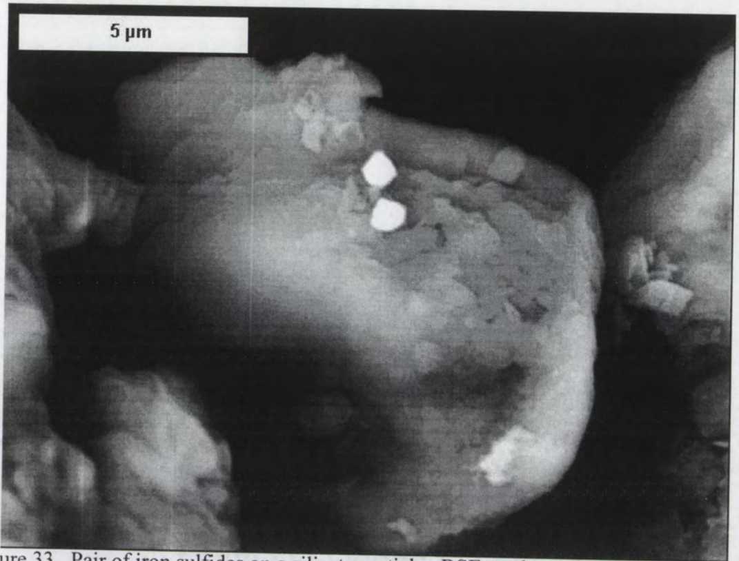
Figure 33. Pair of iron sulfides on a silicate particle. BSE mode, scale bar = 5 \mu\text{m} (sample BLN9-062701-169-182F).
