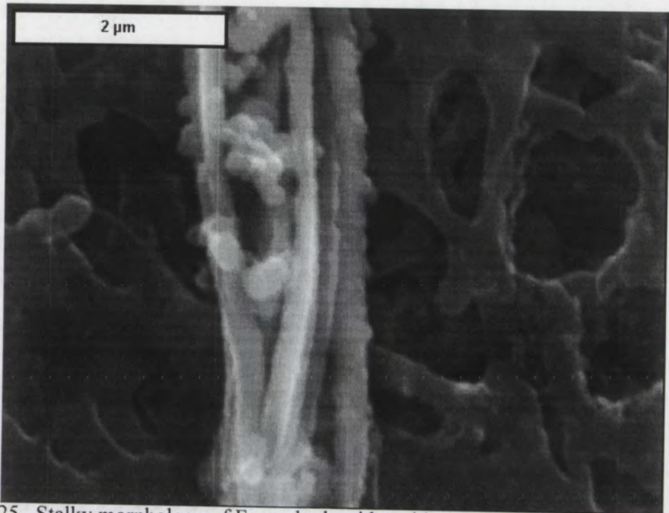
Figure 25. Stalky morphology of Fe oxyhydroxide, with spherical Fe oxyhydroxide between. SE mode, scale bar = 2 \mu\text{m} (sample BLN2-111101-147-156).
