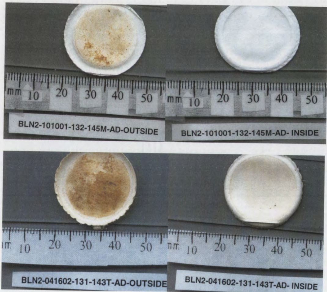
Figure 22. Typical inner and outer surfaces of 0.2 \mu\text{m} cell filters from 10 October 2001 and 16 April 2002.
