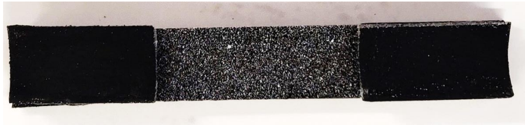
Figure 18 Tabbed specimen prepared with a speckled pattern for DIC
