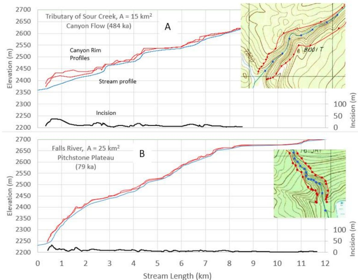
Figure 16. Stream profiles digitized from USGS 7.5' topographic maps (blue) with profiles of the rhyolite bedrock surface measured along the edge of the fluvial canyons (red). Incision between the stream and lower rim in black. Inset topographic maps show profile points mapped on 20-ft contour lines near the flow-margin at the same scale (1-km UTM grid).
