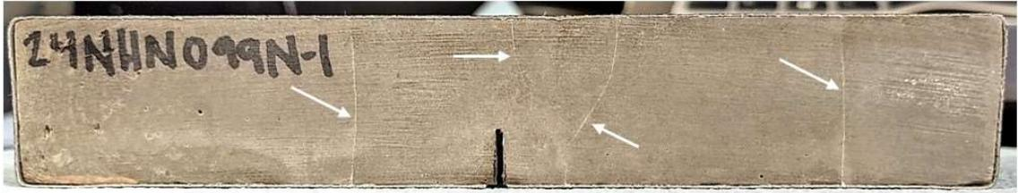
**Figure 50.** Image of calcium leached sample after 20 weeks of exposure, cracks from degradation are pointed out with arrows.
