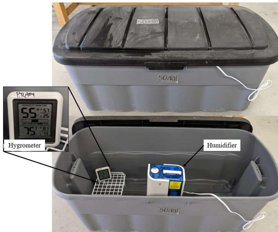
**Figure 11.** Showing the 50%RH chamber which was comprised of a 50-gallon container, rack for samples, humidifier, and hygrometer.
