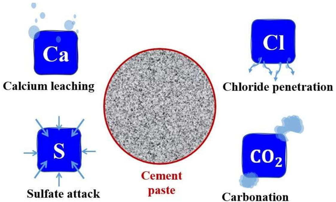
**Figure 2.** Schematic representation of the four primary forms of cement degradation as discussed in this section.
