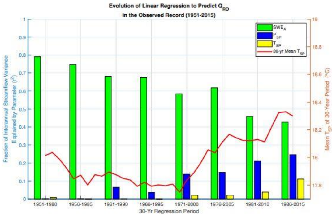
Figure 2 Fraction of interannual variability of Q_{RO} ( r^2 ) (left-hand ordinate) associated with an individual parameter for successive 30-year regression windows. The green bar shows the fraction of interannual variability of Q_{RO} attributed to SWE_A as a first order predictive parameter in the step-wise regression model structure. The blue and yellow bars show the fraction of interannual variability of Q_{RO} attributed to P_{SP} and T_{SP} respectively as second order predictive parameters in the step-wise regressions (step 2 in Table 1). A moving 30-year window with annual resolution is used here to show 30-year mean T_{SP} (shown by the red line with the right-hand ordinate).
