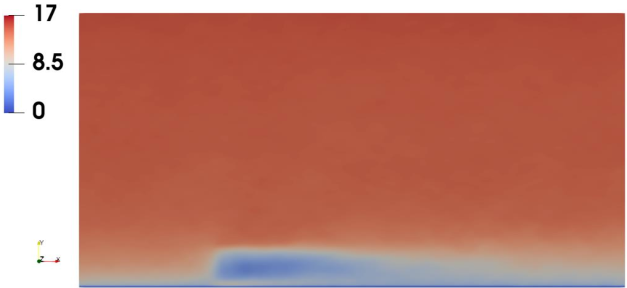
Figure 4.4. Time-averaged contour of streamwise velocity in the XY plane for gap 0.25D cross-sectioned at the centerline of the turbine.
