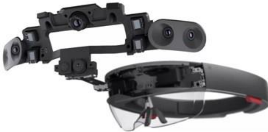
Figure 11. Built-in sensors of HoloLens.
