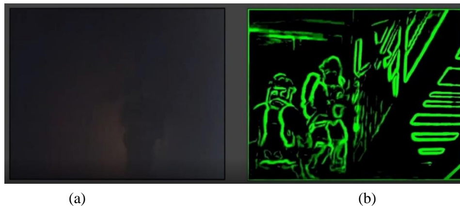
Figure 6. AR-enabled Firefighter helmet called C-THRU produced by Qwake Technologies. (a) Normal Vision. (b) Augmented Vision (Sam J . Cossman et al., 2019).
