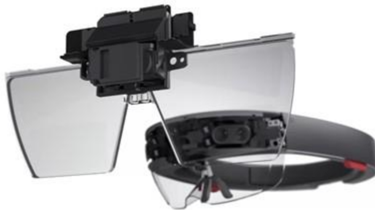
Figure 10. Optical display of HoloLens.
