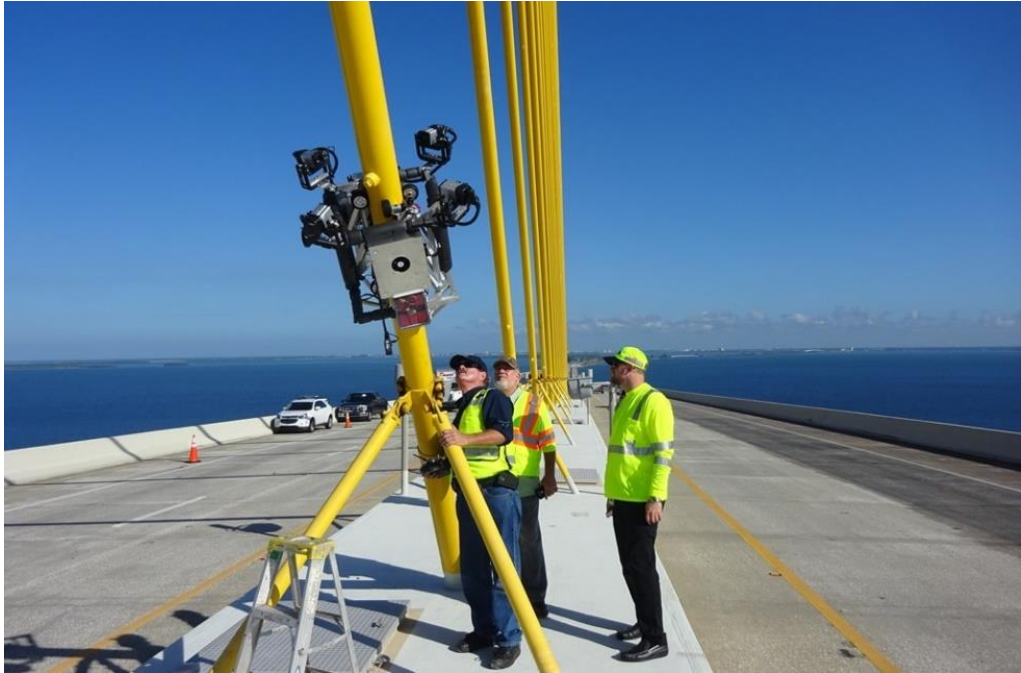
Figure 7. Crawling robots are used in infrastructure inspection where human access is denied (Zasky, 2018).
