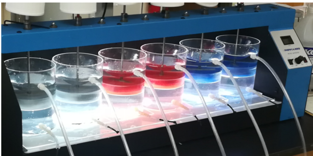
Figure 4-2: 6 of 12 experimental annular bioreactors. P-Methyl = grey cylinders, P-Ester = red, P-Amine = blue.
