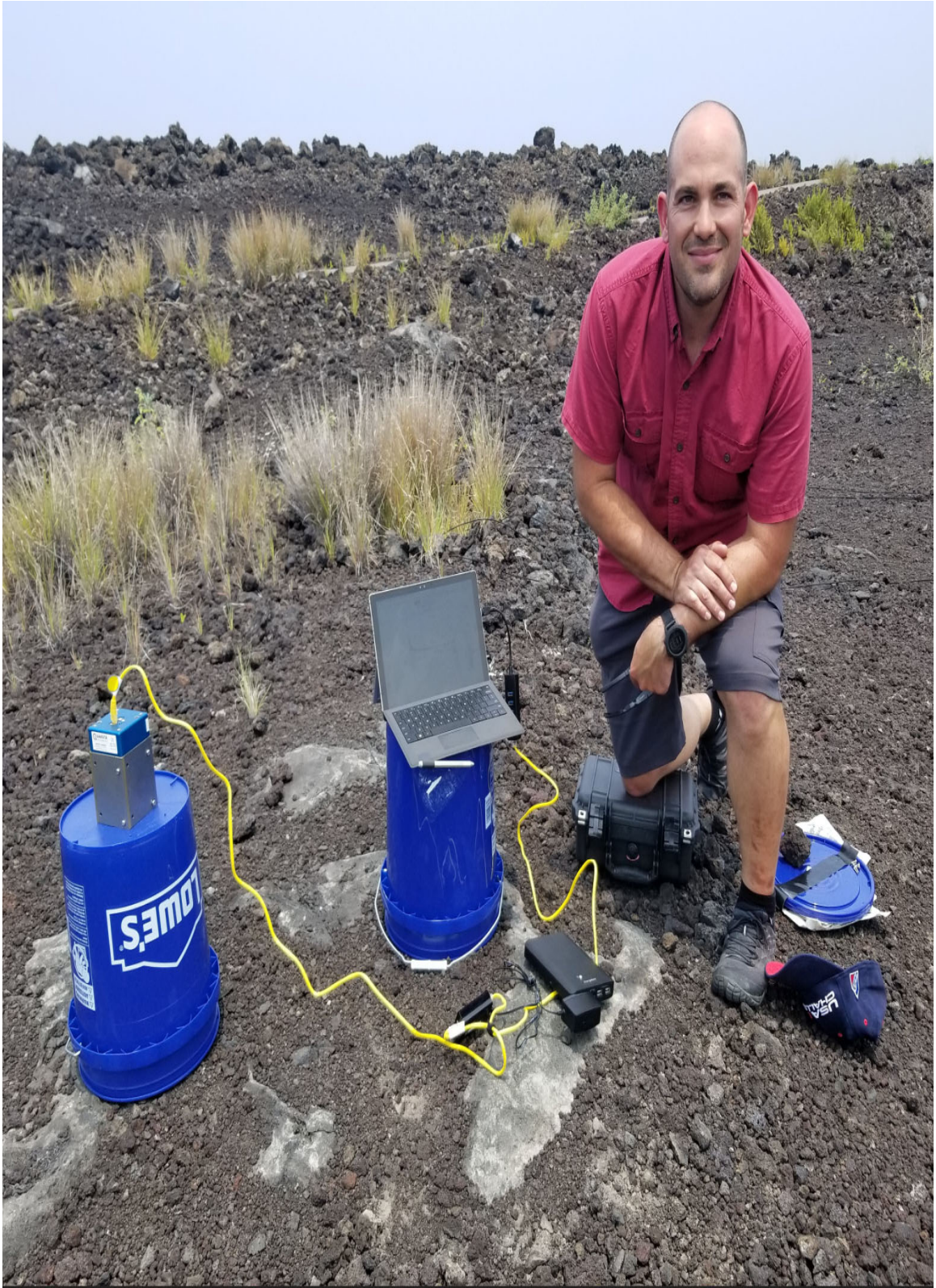
Figure 3-7: Gamma spectrometer and accoutrement used for surveying of Kona basalt and rainfall during heightened Kilauea eruptions
