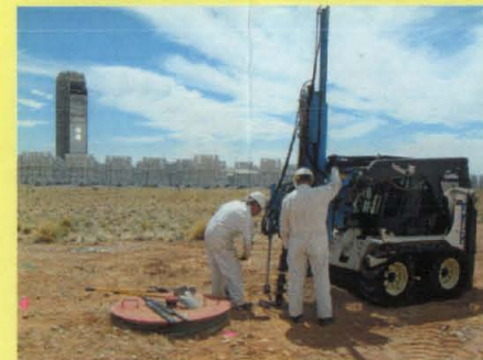
Collecting additional soil samples for VOCs from a borehole drilled adjacent to the seepage pit at AOC 1116 with the Solar Tower in background.
