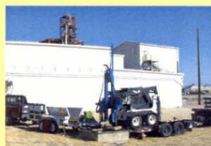
Collecting soil samples with the Geoprobe.
