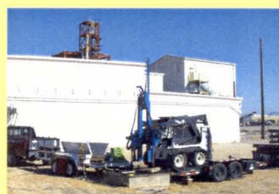
Collecting soil samples with the Geoprobe.
