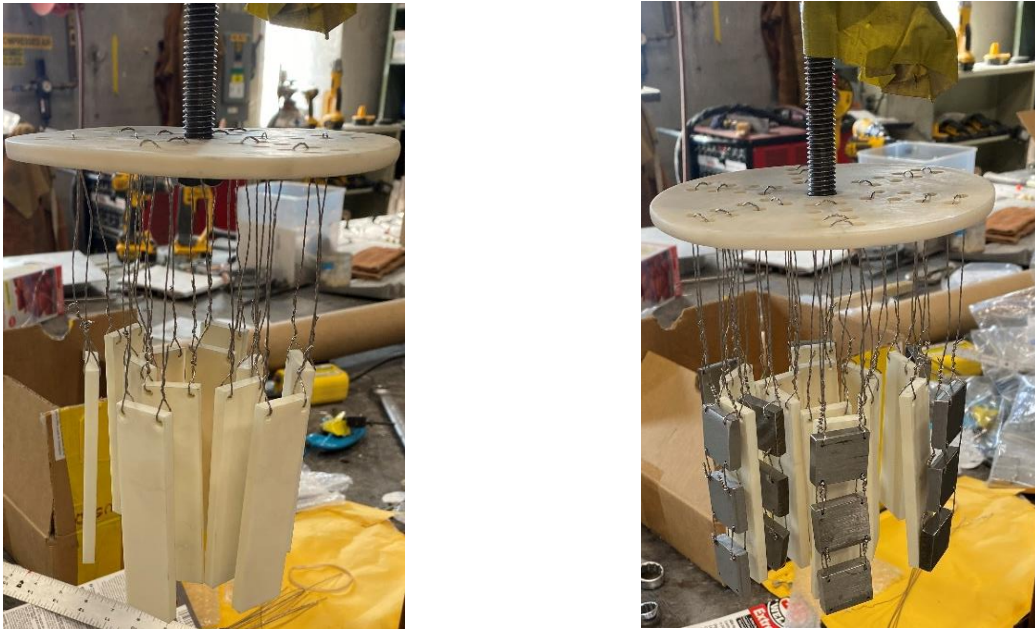
Figure 8: Coupon Sample "Chandelier" with Alumina Spacers, with and without Coupons
