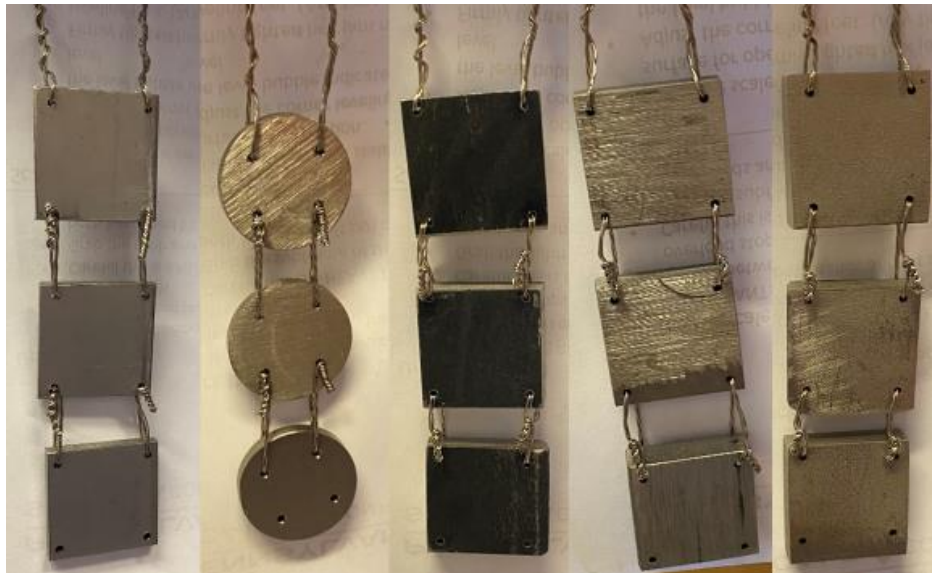
Figure 17: Pre-Test Nickel Alloy Samples left to right: Haynes 230, Haynes 282, Inconel 740H, Inconel 625, Inconel 800H
