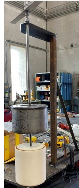
Figure 11: Sliding Rod and Coupon Holder Raised Above and Lowered into Alumina Crucible
