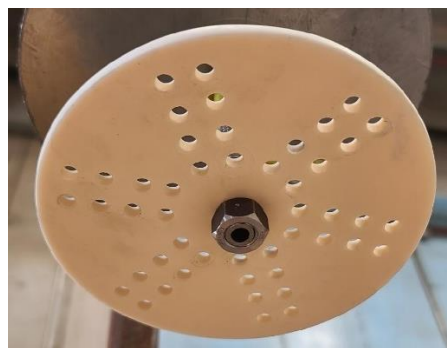
Figure 9: Alumina Coupon Disk Mounted on Threaded C276 Rod
