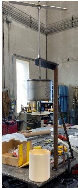
Figure 11: Sliding Rod and Coupon Holder Raised Above and Lowered into Alumina Crucible
