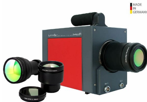
Figure 11: The ImageIR® 8300 hp, using a 100mm lens at a resolution of 640X512 pixel was used to obtain the sets of thermograms.
