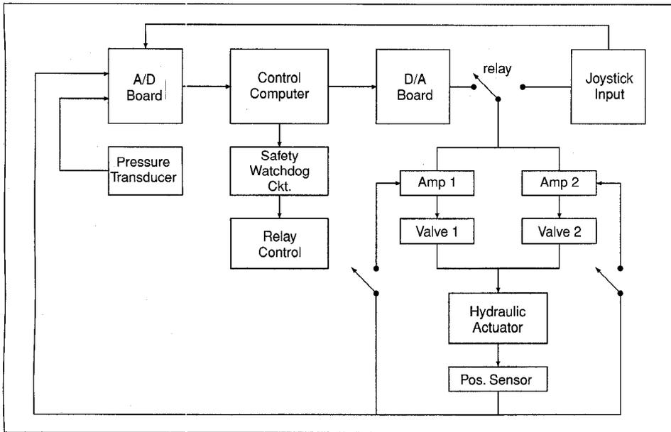
Fig. 6. Block diagram of computer control system.
