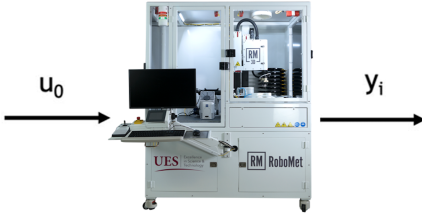
Figure 2: Open loop nature of the Robo-Met.3D™ system, where a set of fixed user inputs, u_0 , form a polishing routine (recipe) that generates an output removal amount y_i which may vary due to system dynamics.
