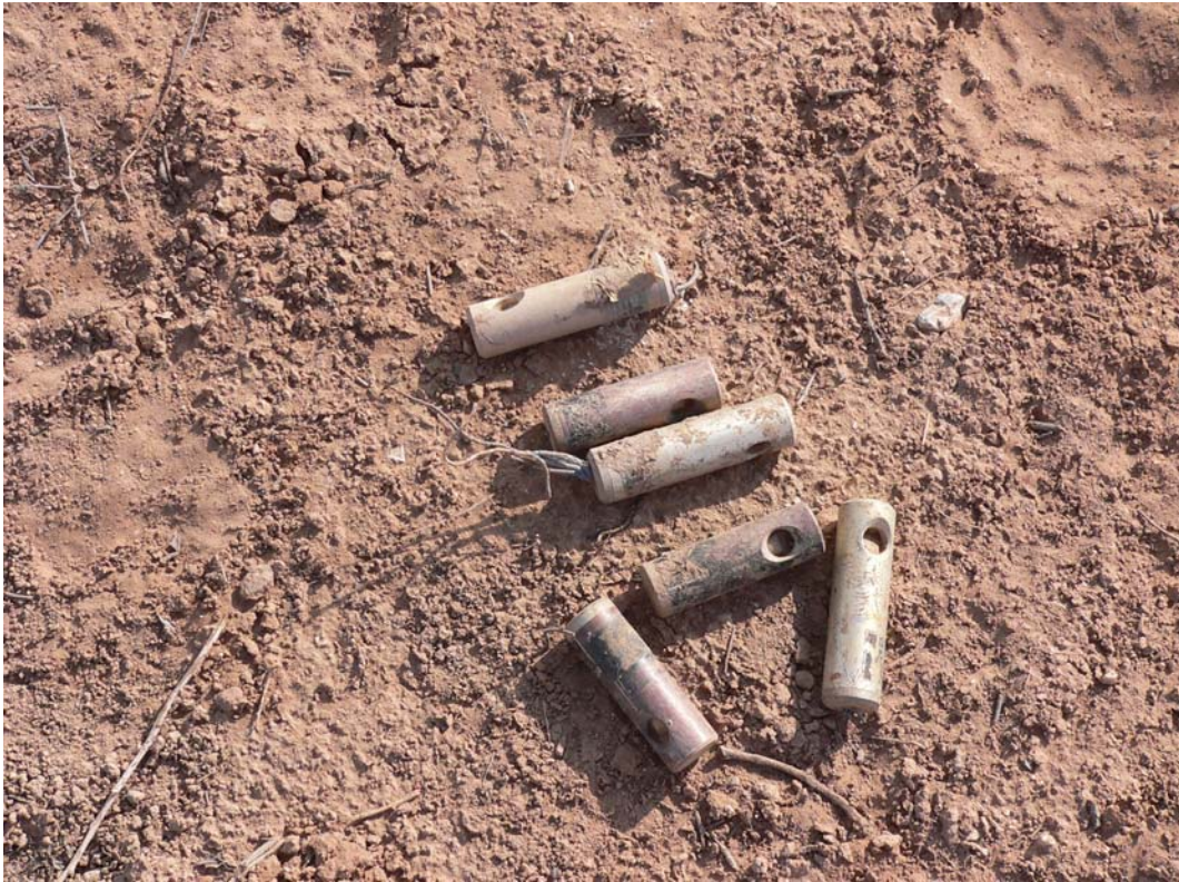
LTES Site 1 Powder Activated Cable Cutters
