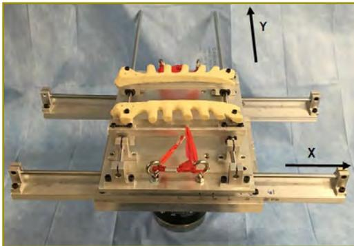
**Figure 1.** Experimental test setup showing sternal halves positioned in the custom designed testing fixture. A force of 15 kN is positioned under the fixture to collect data on applied axial load during closure.
