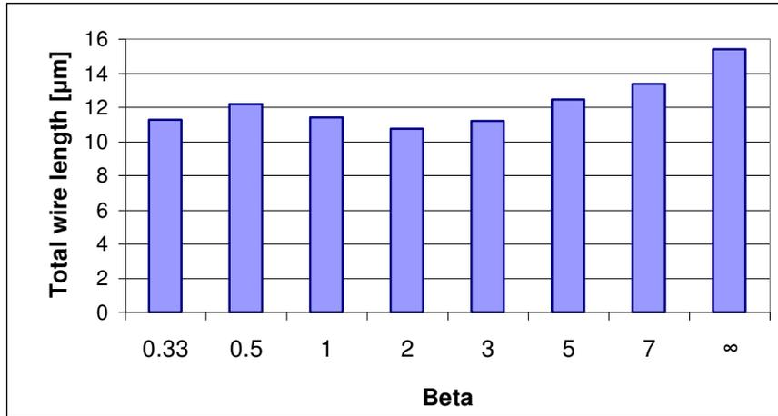
Figure 4.8. Total wire length for generated layouts with different  $\beta$ .
