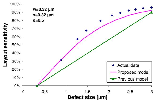
**Figure 3.4.** Comparison of the proposed sensitivity model with extracted layout sensitivity and a previous sensitivity model [41] for short defects.
