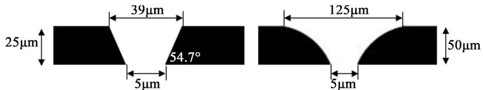
Figure 3.18 –Nozzle outlet shape of (a) MEMS VMA and (b) Metallic VMA.
