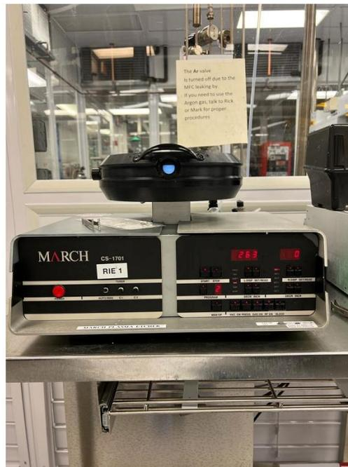
Figure 4.11 March plasma Etcher (Reactive ion etching).
