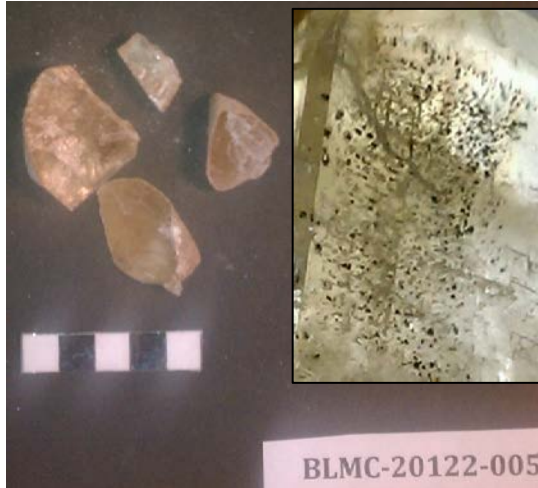
Figure 47: Sample BLMC-20122-005. Calcite spar. Scale bar is in cm. Inset is a backlit close-up of petroleum inclusions in the largest fragment. (Photo Credit: Dave Decker).
