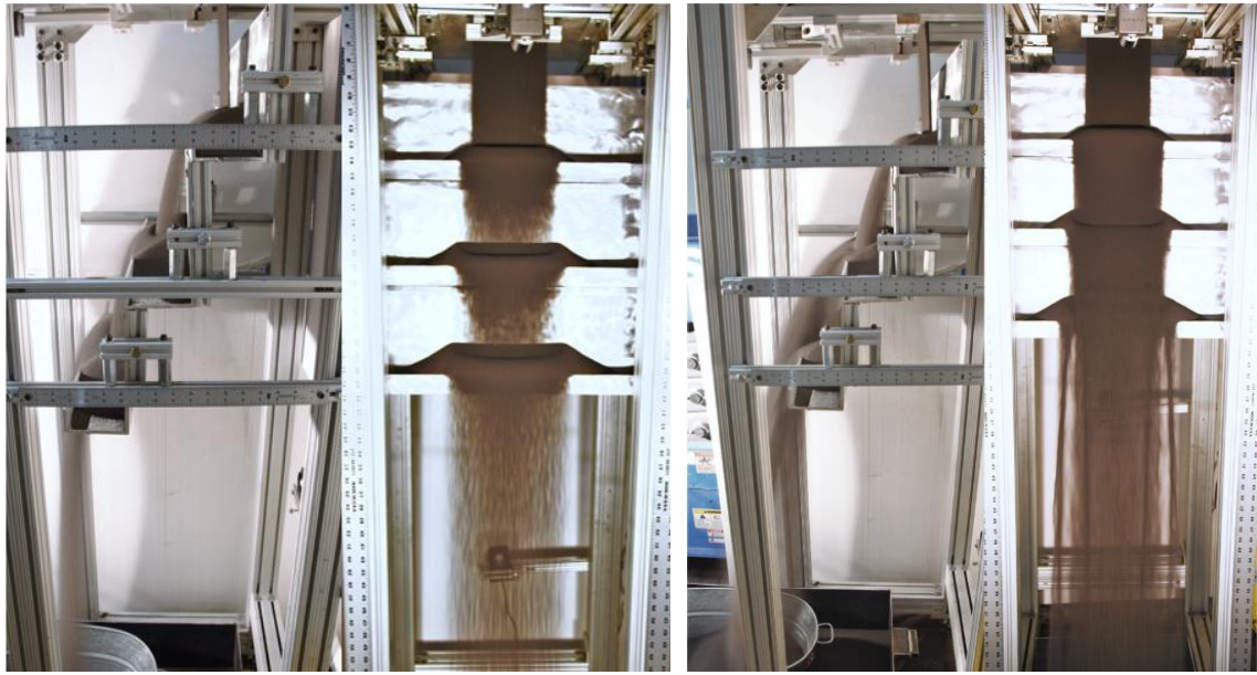
Figure 14: Particle Bounce over 3 troughs. (1) Particle flow over 3 troughs at 4.1 kg/m/s. (2) Particle flow over 3 troughs at 9.8 kg/m/s. Inter trough distances of 8".
