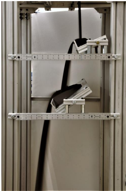
Figure 10: 2 trough configuration with a 4.1 kg/m/s mass flow rate. First trough 65 orientation, on-v position, 12" from curtain origin. Second trough 45 orientation, on-v position, 12" below the first. Particles can be seen bouncing at the second trough.
