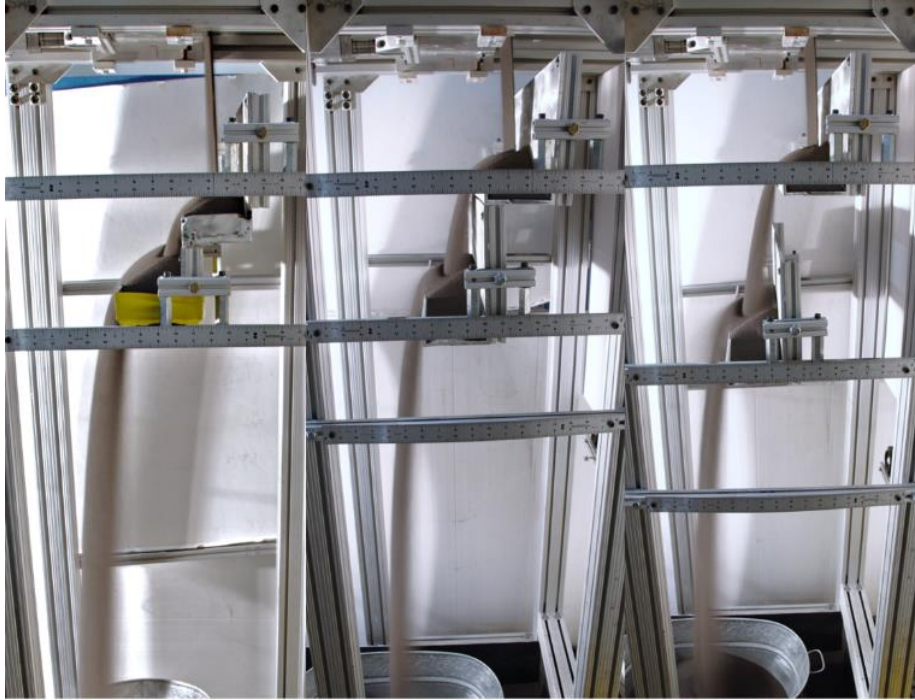
Figure 13: 2 stAIR tests at 4.1 kg/m/s. Inter stAIR distances of 4"(leftmost), 8"(center), and 12" (rightmost).
