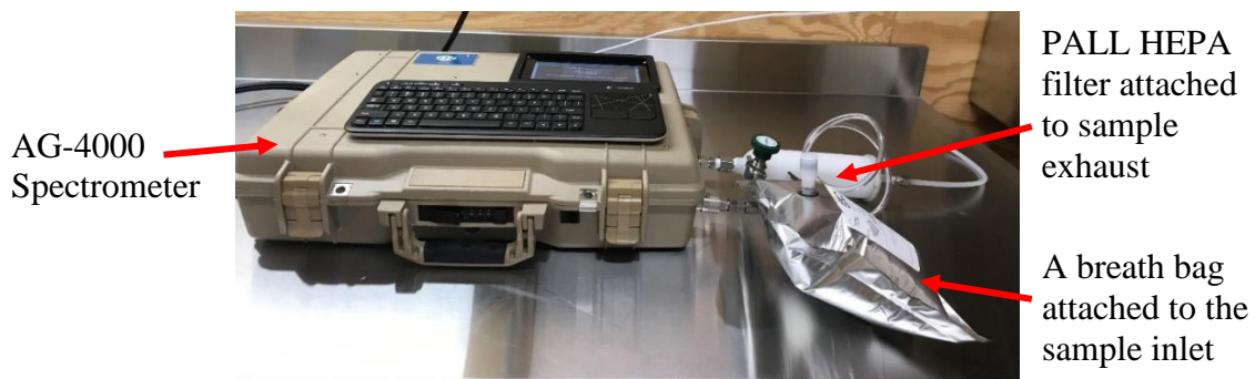
Figure 2.1: AG-4000 Breath Test Assembly RingIR Device with Collection Mechanism
