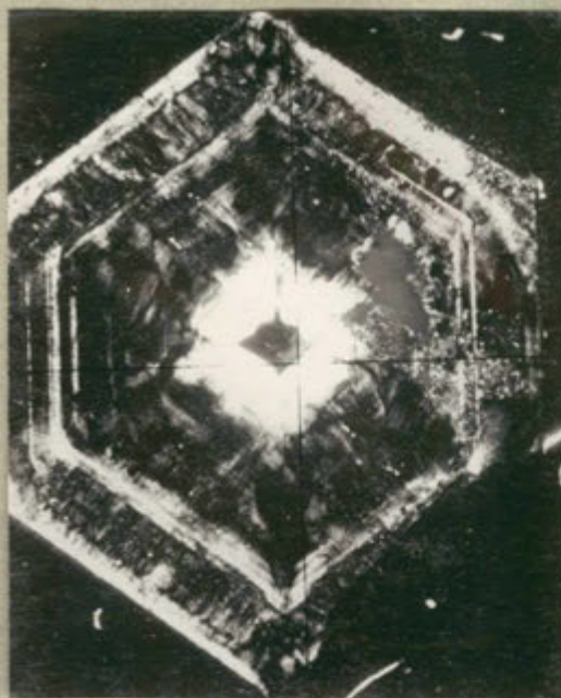
B. Garnet VI.C: Anisotropic crystal, view parallel two-fold axis, after heating for 1 1/4 hours, X-nicols, 28X
