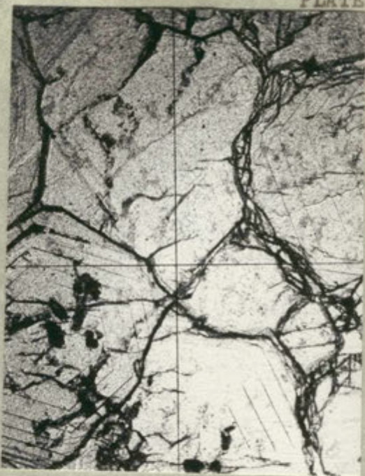
A. Garnet III: Anisotropic crystals, before heating, plane polarized light, 26X
