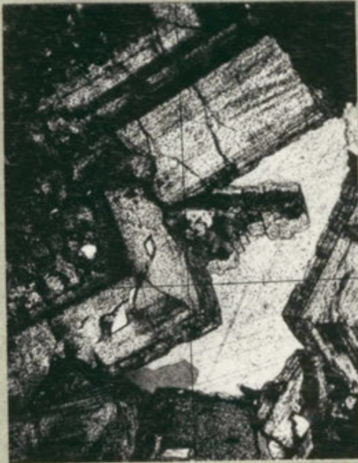
A. Garnet I: Anisotropic crystals, before heating, X-nicols, 80X
