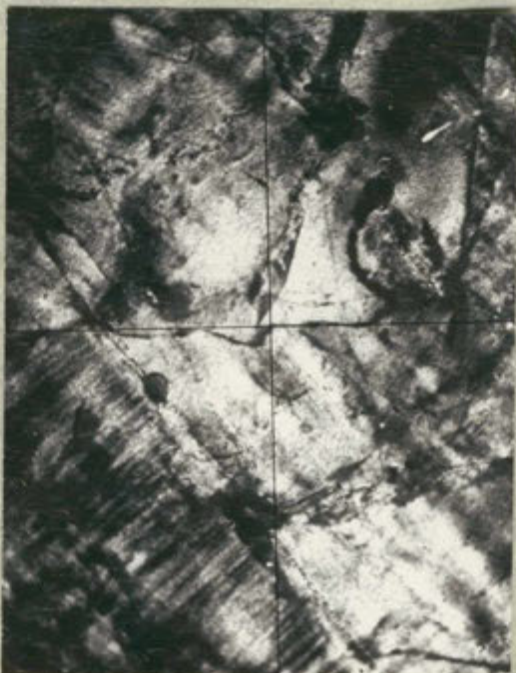
C. Garnet II: Anisotropic mass, before heating, X-nicols, 26X
