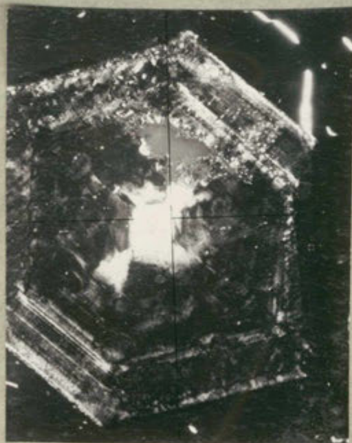
D. Garnet VI.C: Anisotropic crystal, view parallel two-fold axis, rotated 45^\circ from A., after heating for 1 1/4 hours, X-nicols, 28X
