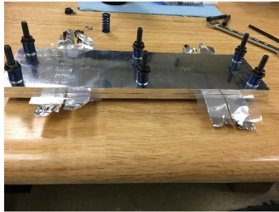
Figure 7. Compression Plate Test Setup with D1 Test Structures
