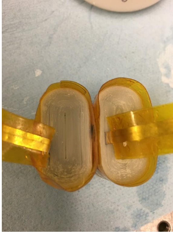
Figure 14. Capacitors with Outside Dam Being Readied for Dielectric to be Placed Inside the Dam
