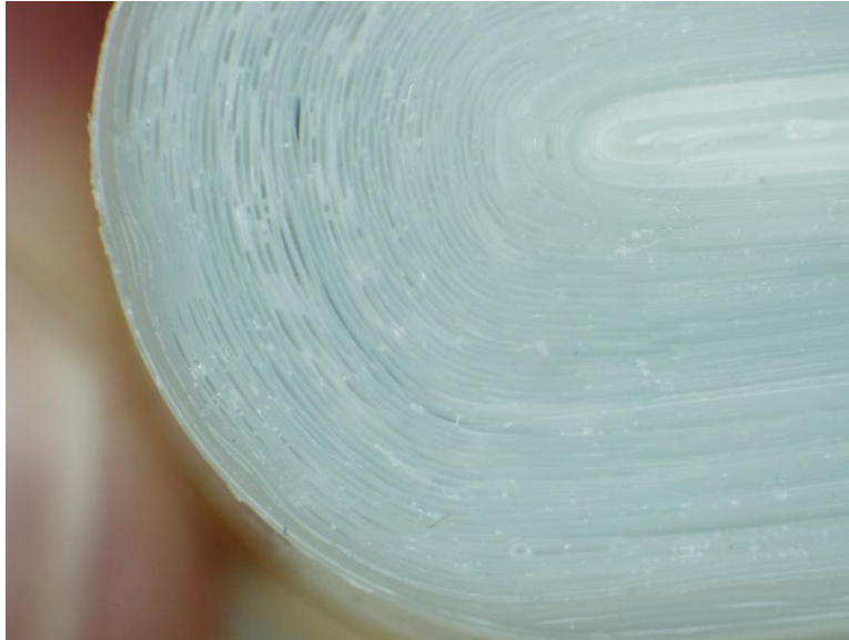
Figure 13. Capacitor Windings After Being Pressed and Annealed
