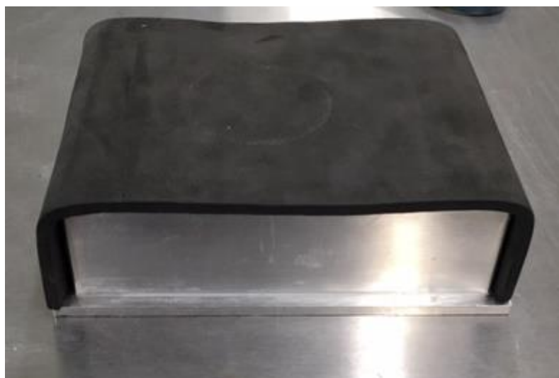
Figure 25. Aluminum block with Foam Used After Determining Film Thickness was Independent of Speed and Pressure
