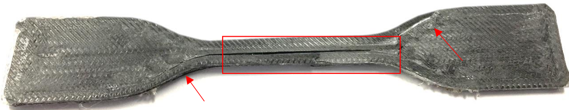
Figure 21. Fractured sample (Type II) exhibiting inter-filament failure. Box contains the longitudinal matrix crack and arrows point out the crack initiation points.
