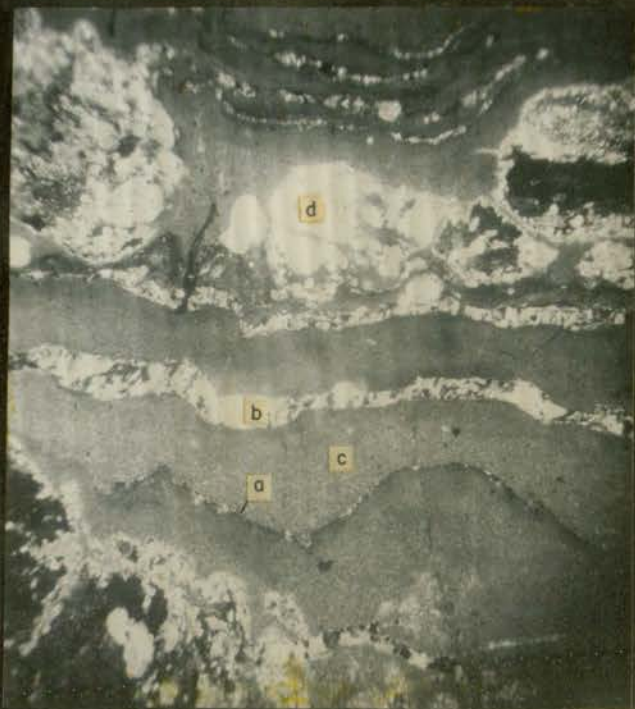
Figure 14. Photomicrograph of transition zone (crossed nicols); a, organic lamina; b, fibrous gypsum; c, microcrystalline limestone; d, gypsum nodule lined with calcite crystals and quartz grains. Scale 0.5 mm. Sample obtained from locality 2 (Fig. 5).
