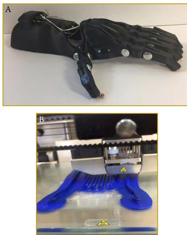
**Figure 1.** (A) 3D-printed Cyborg Beast prosthetic hand by e-NABLE, printed in our laboratory. (B) Cyborg Beast during printing with the Ultimaker 2+ Extended printer using blue acrylonitrile-butadiene-styrene polymer.
