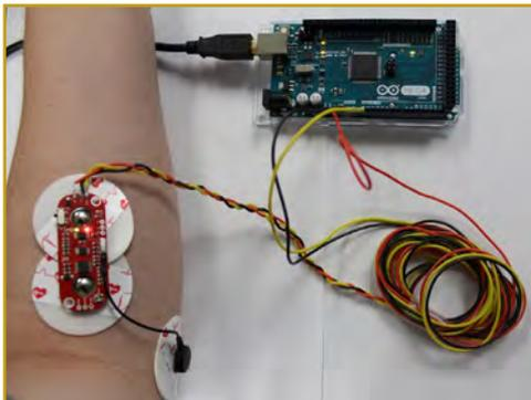
**Figure 5.** Myoware sensor attached to an arm and connected to an Arduino MEGA microcontroller.
