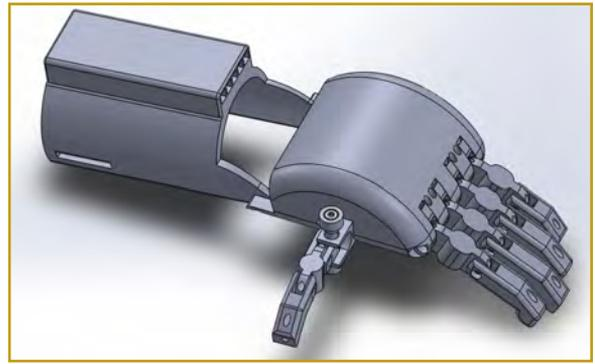
**Figure 3.** First iteration of the Cyborg Beast re-design, which protects the exposed “tendon” cables from early failure. Notably, there is a greater level of coverage of the cables as compared to Figure 1. Additionally, the thumb is modified to allow for manual repositioning of the angle of the thumb relative to the fingers to allow for better opposition as preferred by the user.
