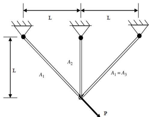
Fig. 2 Design of three bar planer truss
