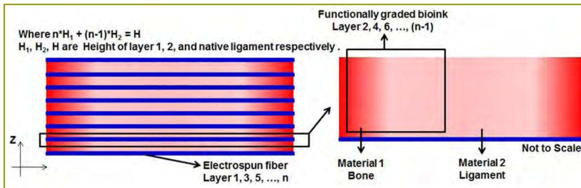
Figure 6. Schematic representation of the (Left) hierarchical and (Right) functionally-graded composite scaffold targeted with this technology.
