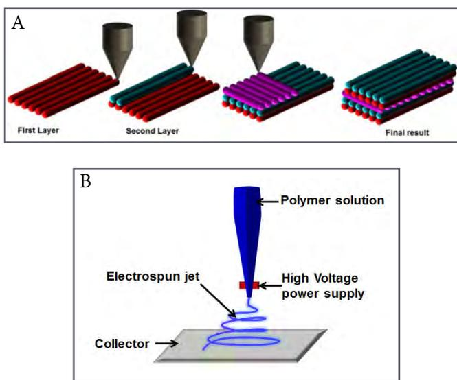
**Figure 1.** (A) Representative example of 3D bioprinting using multiple bioinks deposited from their respective syringe deposition systems. (B) Representative schematic describing the primary characteristics of an electrospinner.
