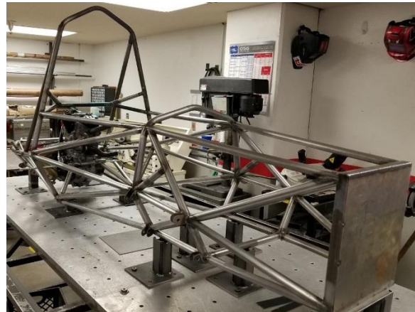
Figure 48. Fabricated chassis front view
