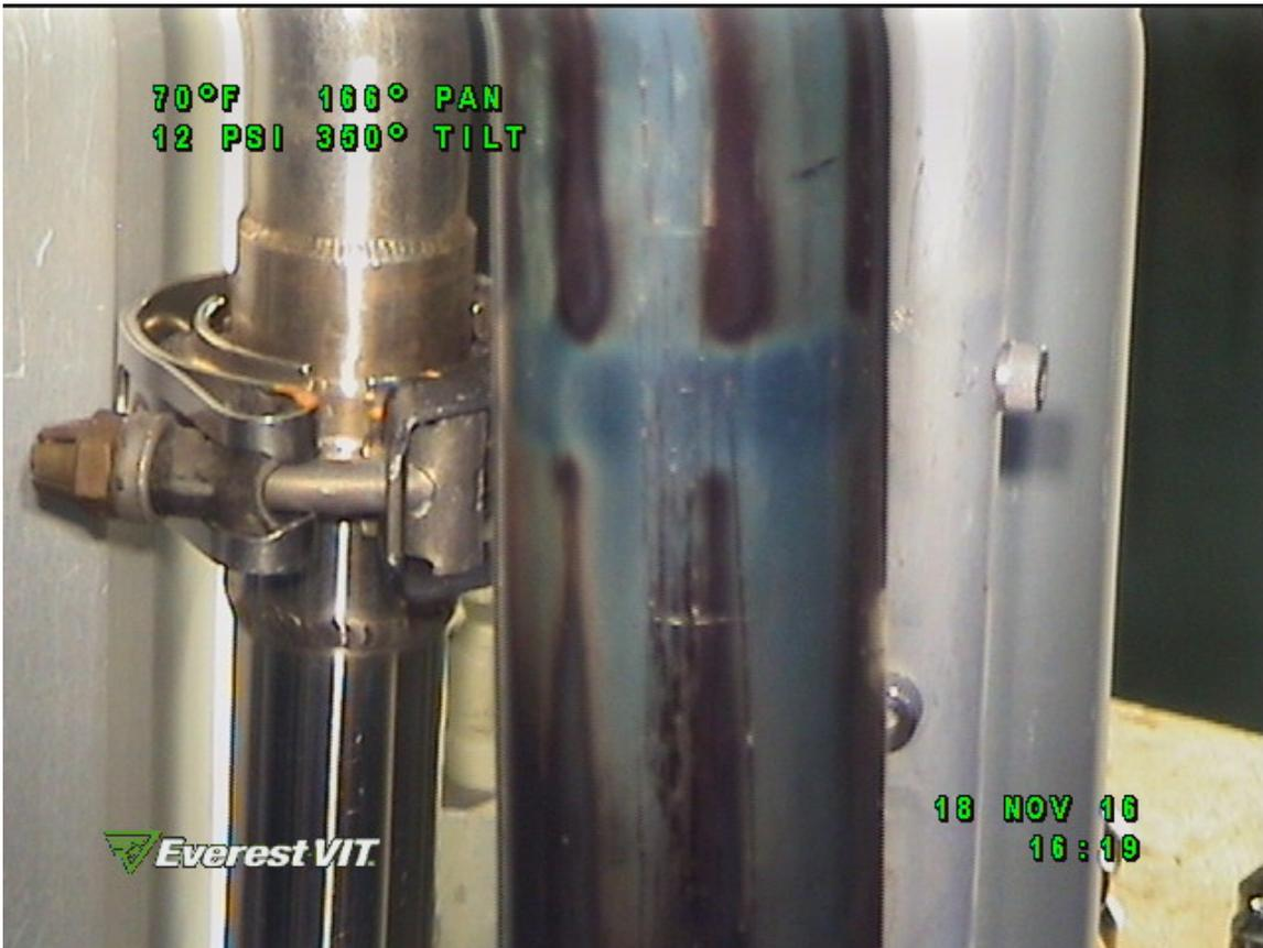
Figure 5.24: Photograph of the outer surface of the cladding of a fuel element in the ACRR.
