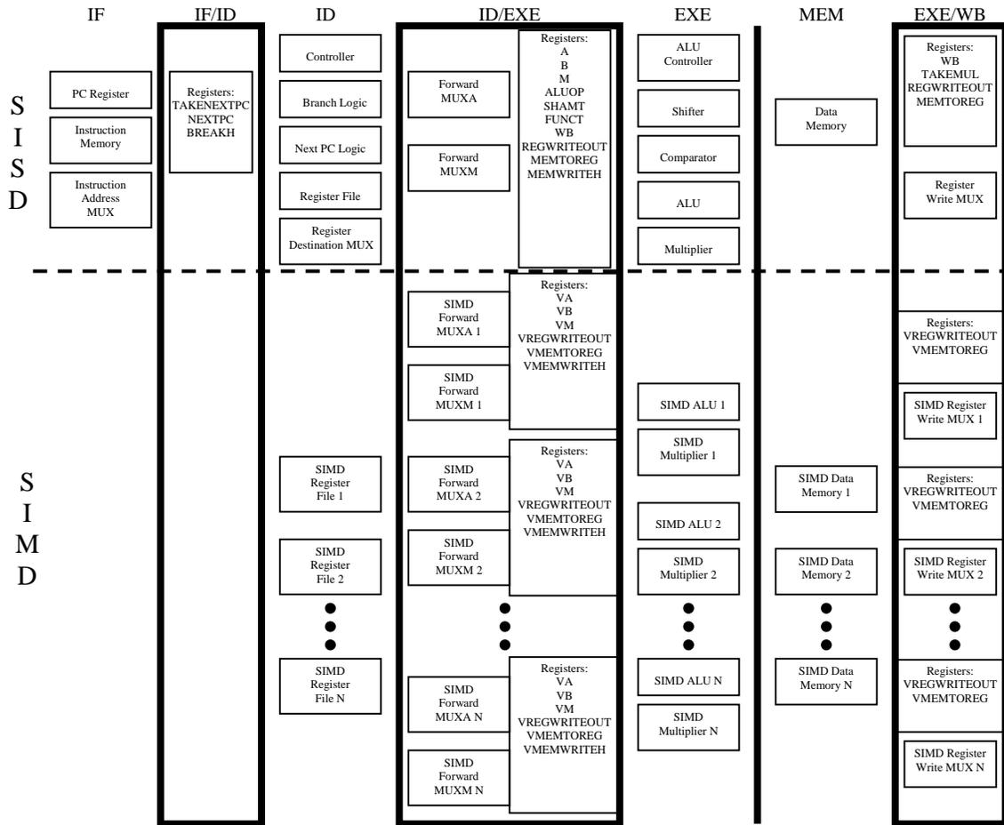
Figure 17: SISD and SIMD Block Diagram of Processor.
