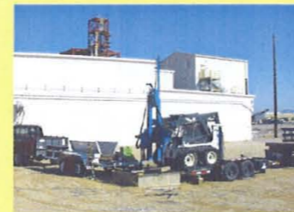
Collecting soil samples with the Geoprobe.
