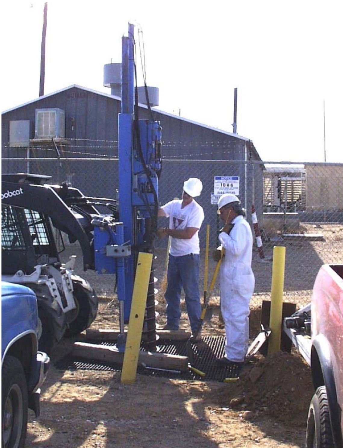
Figure 3.3-1 Collecting soil samples with the Geoprobe™ at DSS Site 1086 seepage pit. View to the east. September 6, 2002
