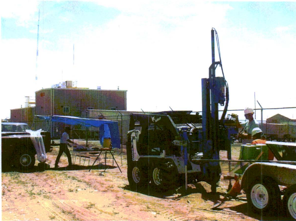
Figure 3.4-2 Collecting soil samples with the Geoprobe™ in the DSS Site 1079 drainfield at Building 6643. View to the southwest. August 22, 2002
