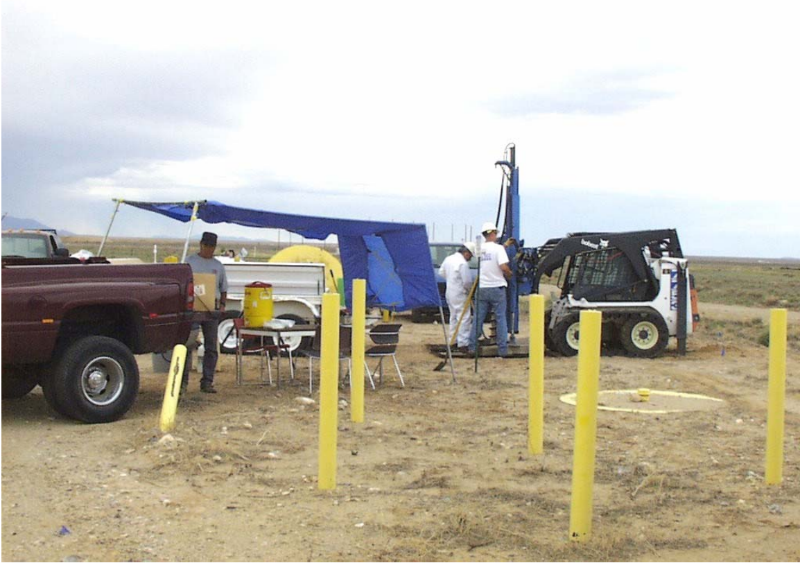
Figure 3.4-1 Collecting soil samples with the Geoprobe™ at DSS Site 1081, Building 6650 Septic System. View to the south. August 29, 2002
