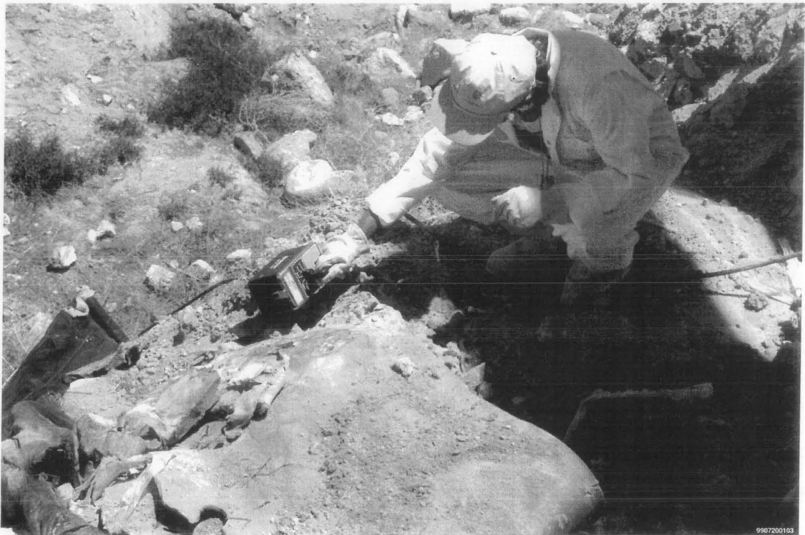
Figure 3.4.5-2 July 1998 photograph with a Radiological Control Technician surveying SWMU 228A weapon debris at Scrappy-DU with a Bicron \mu rem radiation meter. The weapons debris consists of black rubber pads and yellow DU fragments.
