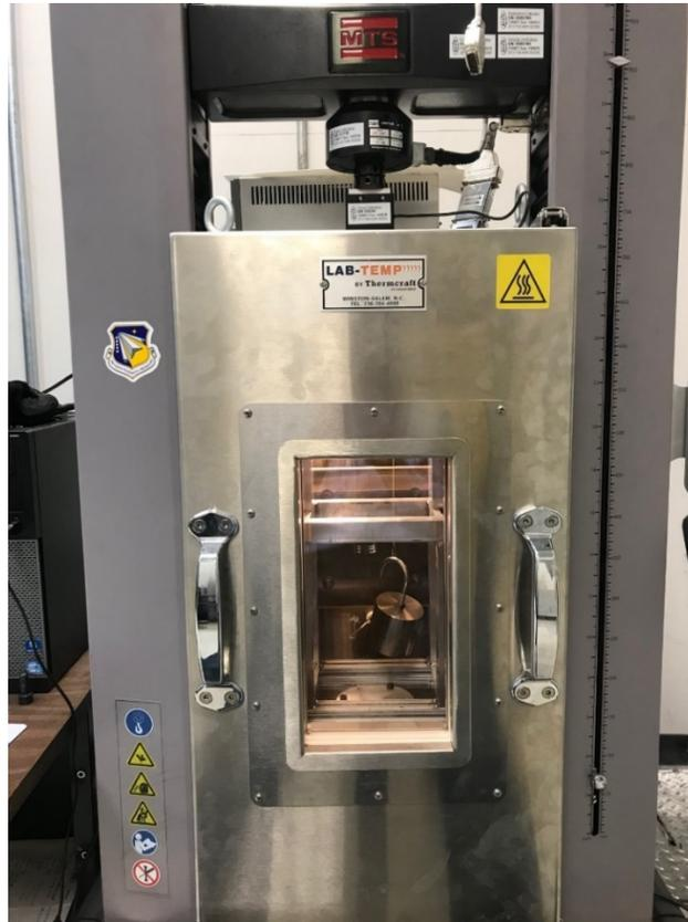
**Figure 3.14 Lab-Temp Thermal Chamber**
