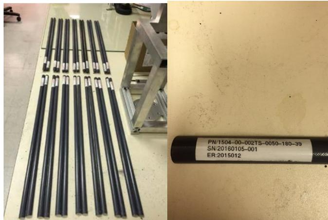
**Figure 3.15 Control Group Tape Springs for Structural Testing**
