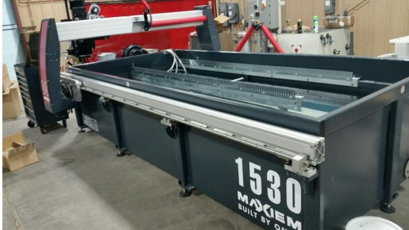
**Figure 3.10 Waterjet Cutting Machine at Holloman Air Force Base**
