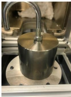
**Figure 3.20 Counter Mass for Tape Springs’ Structural Testing**
