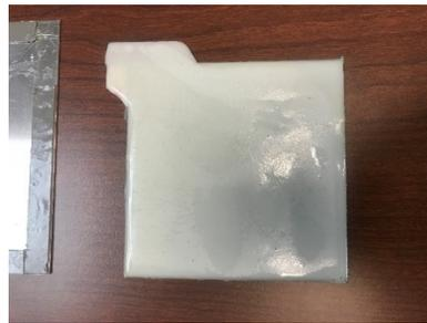
**Figure 3.8 Neat Epoxy Sample #2**
