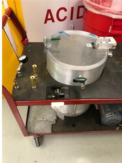
**Figure 3.5 AFRL's De-Gassing Chamber**
