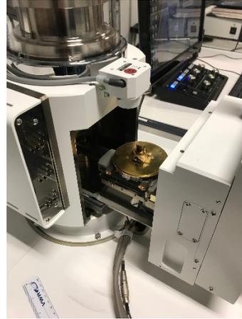
**Figure 3.34 JEOL-JSM-IT100 SEM/EDS for ANP Dispersion Examination**
