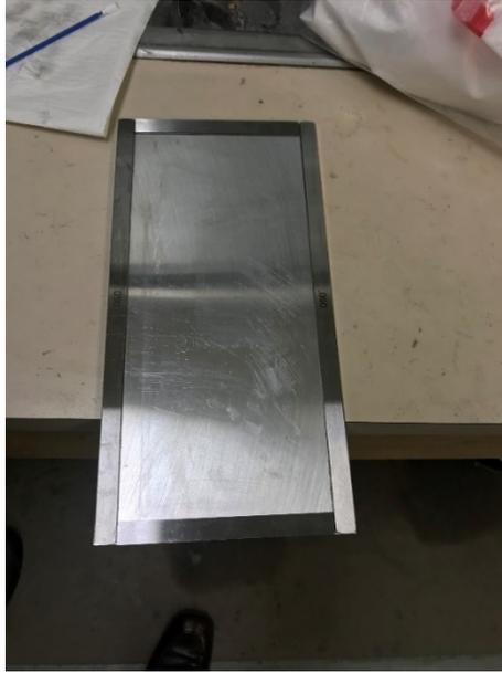
**Figure 3.6 Mold for Neat Epoxy Sample**
