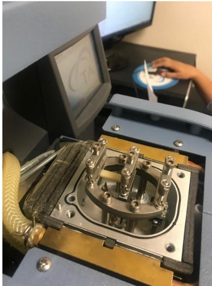
**Figure 3.27 DMA Testing of ANP Coupons**
