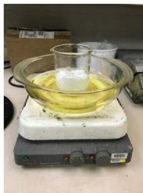
**Figure 3.4 Preparation of Neat Epoxy**
