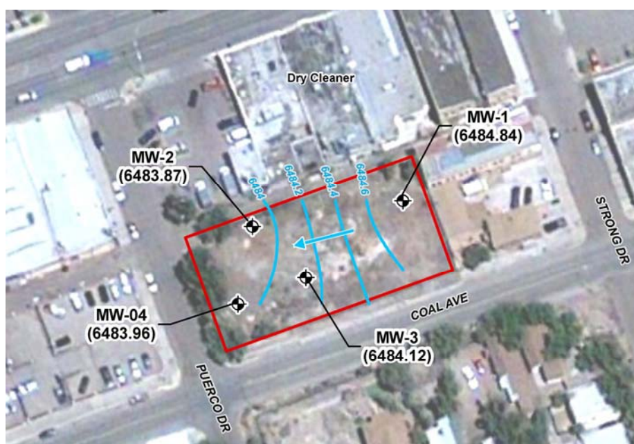
Figure 5: Groundwater Monitoring Wells and Potentiometric Surface with Elevations (INTERA, 2012)
